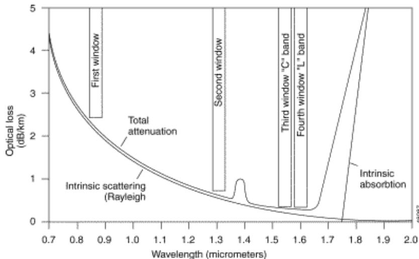
**Fig. 3:** Attenuation curve and transmission windows used in fiber optics communications. Very reliable and long lifetime electronic components were developed for these specific wavelength ranges to fulfill the stringent component lifetime requirements of the telecommunications industry. (Illustration from Cisco web page: [http://www.cisco.com/univercd/cc/td/doc/product/mels/dwdm/dwdm\\_ovr.htm#xtocid629215](http://www.cisco.com/univercd/cc/td/doc/product/mels/dwdm/dwdm_ovr.htm#xtocid629215))
