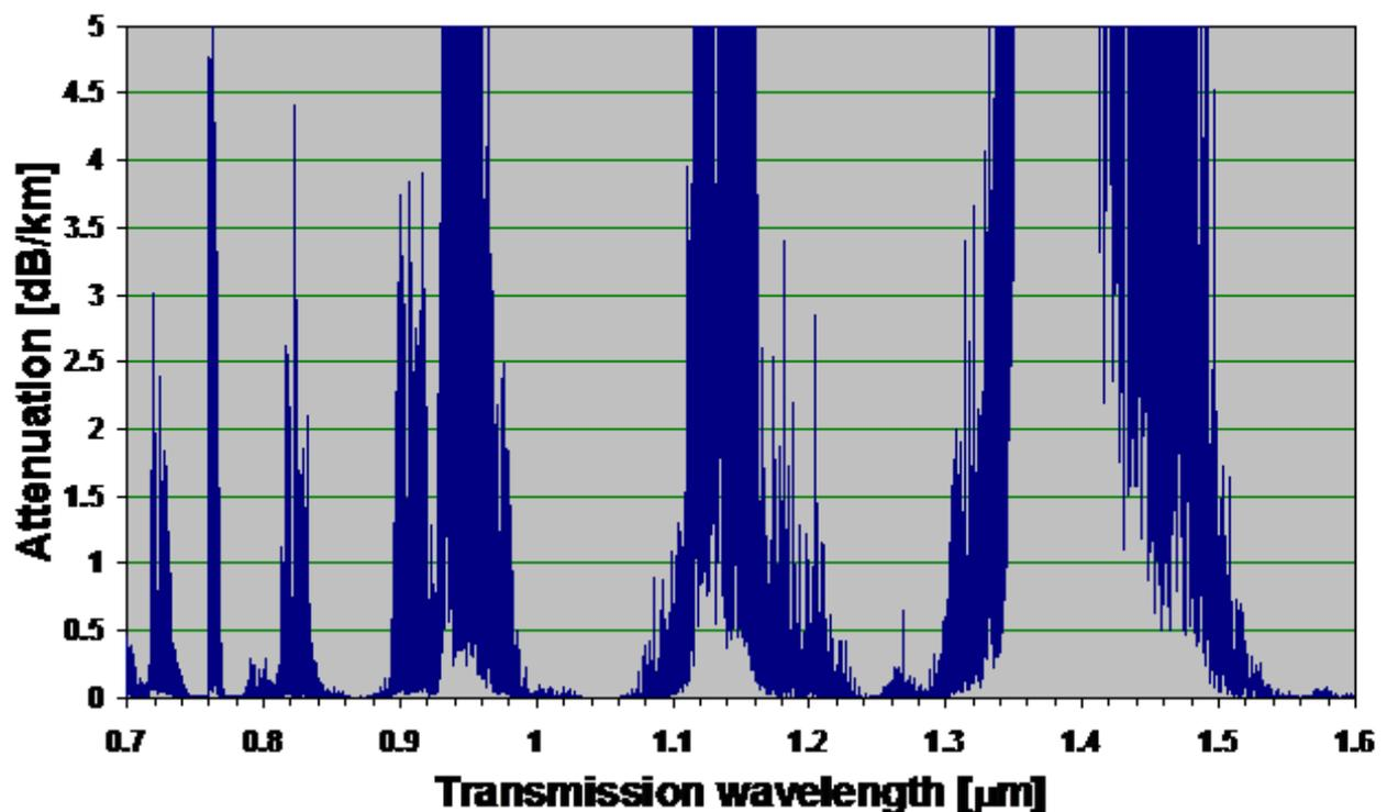
Fig. 1: *Transmission properties of the atmosphere in the near infrared wavelength range under clear weather conditions (visibility > 10 miles). The calculation was done by MODTRAN, a software program developed by the Air force Research Laboratory.*
