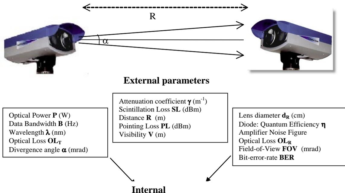
**Fig. 6:** Schematic explanation of internal and external FSO system design parameters.
