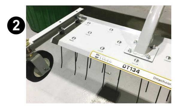
Install the DT Series Dethatcher attachment and lower to the operating position.
