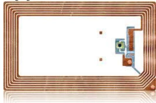
Fig.3: RFID tag inner view
