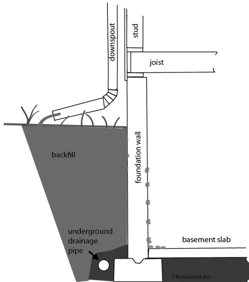
should not have any low-lying areas, but should be sloped so that water will not collect and puddle there. Settled backfill allows water to collect next to the foundation wall
