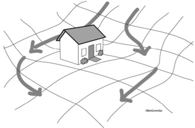
Each drain should have piping that connects it to a storm water drainage system (if there is one), or that drains to either a discharge at a lower grade or into a sump pit that collects and discharges the water away from the building.
