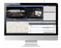
KP1S makes constant recordings of video footage and drive data on a loop as the journey continues. This data can be accessed manually at any time by retrieving the KP1S' SD card(s) and inserting into your PC. The included analysis software allows you to view recorded video and drive data evidence of an event. KP1S does not require 3G or WiFi to operate as a stand-alone system.
