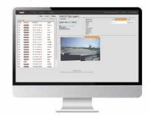
SmartMail was developed with the small/medium fleet operator in mind. It delivers driver safety and protection information to you within moments of an incident taking place. Using KP1 with a cellular modem, safety-critical road events will automatically transmit an email notification with the video clip and event information enclosed. An online portal is provided to help manage all vehicle events.
