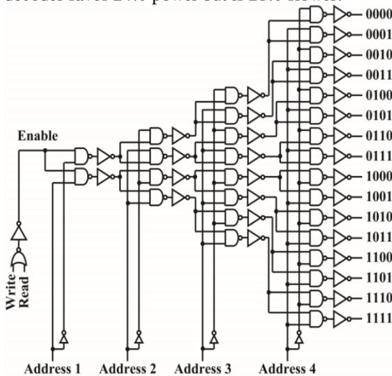
Fig.5: Schematic of the Binary tree decoder
