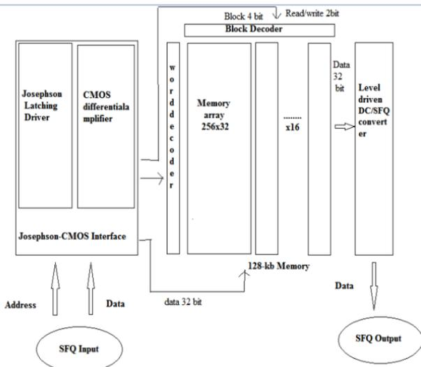
Fig.1: Block diagram of 128 kb Josephson CMOS hybrid memory system
