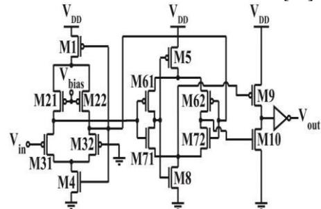
Fig 3 Schematic of the CMOS Differential Amplifier The transistor widths are M1, M21-M32, M4, M5 M61-M62, M71-M72, M8, M9 and M10 are 12.60 um, 10.72um, 9.12um, 7.20um, 8.76um, 9.12um, 1.44um, 4.08um, 0.60um, and 0.46um respectively.
