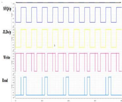
Fig.8: Waveform of 128 kb CMOS Josephson Hybrid memory system using single ended 8T SRAM
