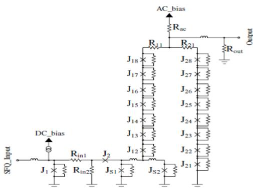
Fig 2 Schematic of Josephson latching driver
