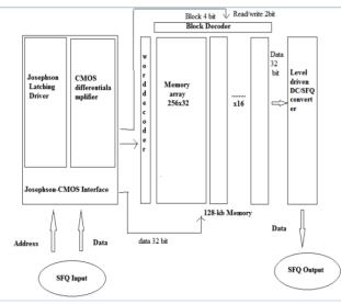
Fig.1: Block diagram of 128 kb Josephson CMOS hybrid memory system
