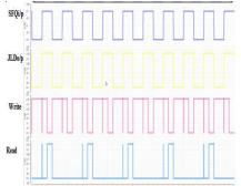
Fig.8: Waveform of 128 kb CMOS Josephson Hybrid memory system using single ended 8T SRAM
