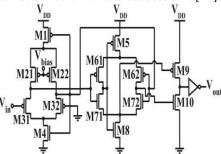
Fig 3 Schematic of the CMOS Differential Amplifier The transistor widths are M1, M21-M32, M4, M5 M61-M62,M71-M72, M8, M9 and M10 are 12.60 um,10.72um, 9.12um,7.20um, 8.76um, 9.12um, 1.44um,4.08um,0.60um,and 0.46um respectively.
