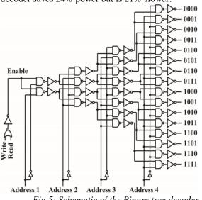
Fig.5: Schematic of the Binary tree decoder
