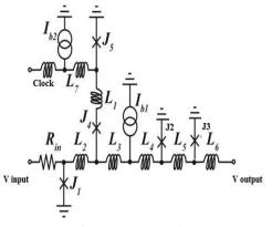
Fig.6: Schematic of the Josephson current sensor (level driven DC/SFQ converter)
