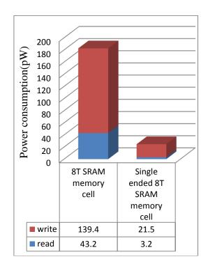
Fig.9: The power consumption chart for 64kb and 128 kb SRAM Memory cell
