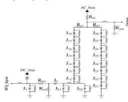
Fig 2 Schematic of Josephson latching driver
