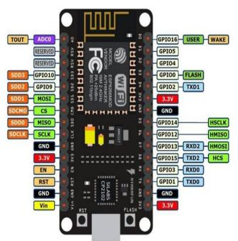
Fig 3: Node MCU (ESP8266)
