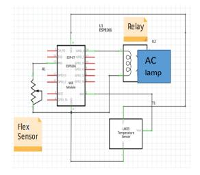
Fig 2: Schematic diagram of Cloud-Based Remote Monitoring Applications with WSN
