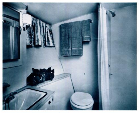
This head is actually a bathroom. It has a stand-up stall shower with curtain; a vitreous lavatory with hot and cold water pressure system. In the vanity locker there are over 4 cu. ft. of storage space. Behind the medicine cabinet are 3 cu. ft. of storage space. There is a screened portlight. Entrance to this head is from the companionway and from the master stateroom. One 110-volt duplex outlet.
