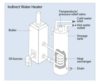
Indirect systems can be fired by gas, oil, propane, electric, solar energy, or a combination of any of these. Tankless systems are typically electric or gas-fired. Also, these integrated or combination water heating systems not only can work with forced air systems but also with hydronic or radiant floor heating systems.
