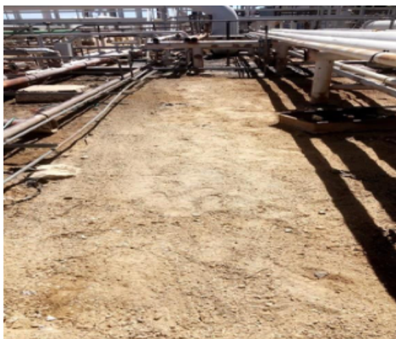
FIG. 6 – TWENTY-FOUR (24) HOURS POST TREATMENT WITH R3MEDIATE. WEST TEXAS GAS PROCESSING PLANT. HYDROCARBON RELEASE WITH SOIL, PIPE & GRAVEL STAINING. (R3ICS, LLC 2019 JULY)
