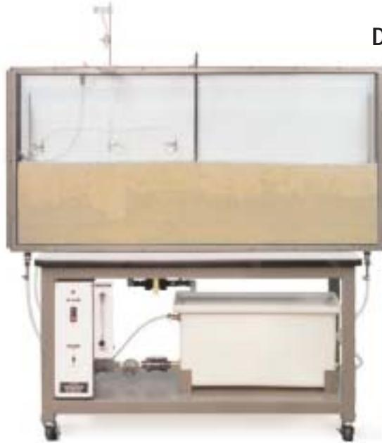
**Model H-6510** Drainage and Seepage Tank Demonstrator shown with sand (not supplied)
