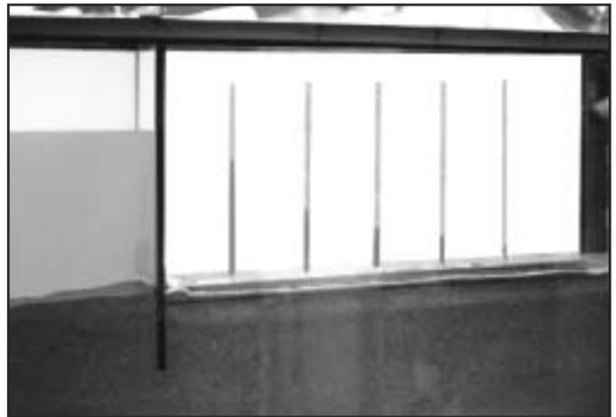
**Purpose:** To 1) demonstrate direct pressures acting to uplift a retaining structure, and 2) construct a flow net.
