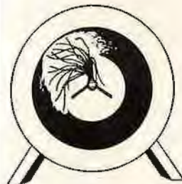
Tracer will lie down in flight and fluff out on impact at target.
