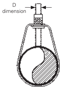
Adjustable swivel Ring - rod tight to pipe
