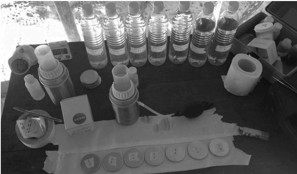
Figure 8. Bacteriological testing using membrane filtration. Photo by author
