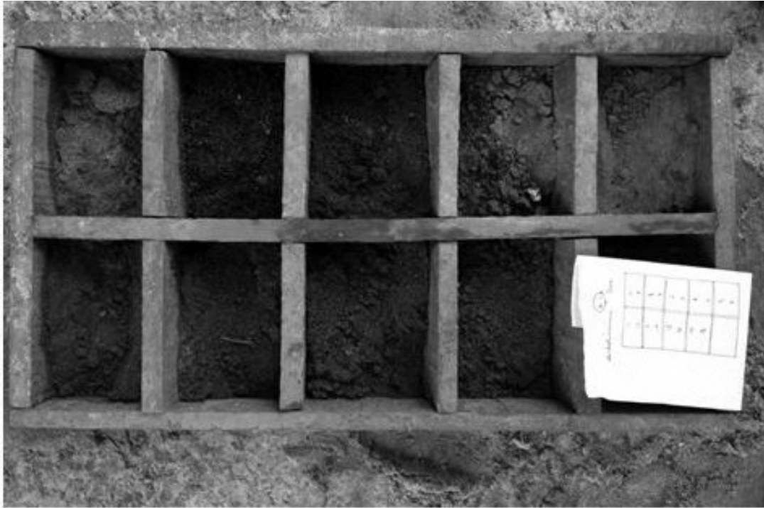
Figure 6. Madrill sample box used for collecting soil samples from the drill slurry. Photo by author
