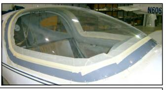
Note: Canopy frame must be fitted to the fuselage, canopy tip up support arms installed, overhead latch installed, cockpit side location tabs installed, and gas strut ball ends in place. This task is best done before the firewall and pedal assemblies are in place, this allows you to crawl in the front and clean up the glue which will come out around the flange.
