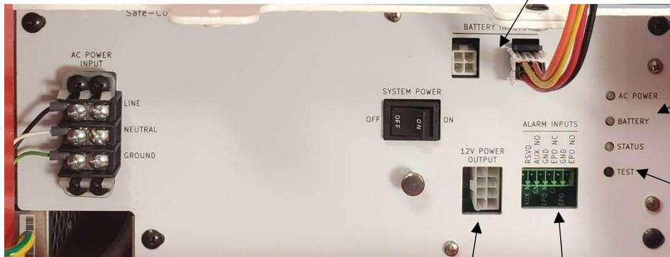
Indicator LEDs display the status and alarms of the BBU.
