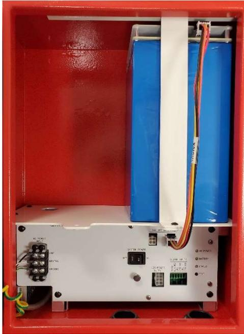
Internal view with one battery pack installed.
