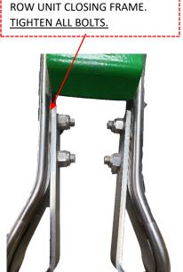
ENSURE THAT THE BRACKETS ARE LEVEL ON THE TUBES AND
