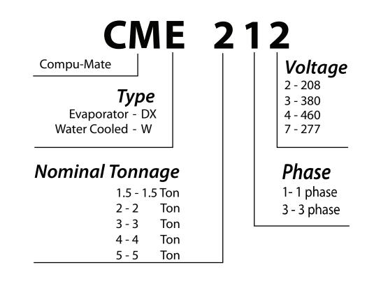
The Compu-Mate units DX systems are suitable for non-ducted application designed for indoor wall and floor mount evaporator section with a matching outdoor condensing unit. Available condensing units: **CFCU** Air Cooled Centrifugal Fan Condenser Unit **PFCU** Propeller Fan Condensing Unit **WCCU** Water Cooled Condensing Unit
