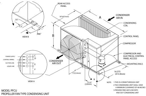
3-PROVIDE FREE AIR FLOW INTO AND OUT CONDENSING UNIT
