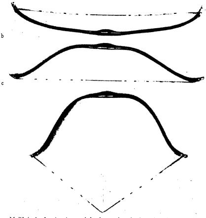
a, Modified grip of an American-made longbow to show the change in midsection from that of the English longbow. The midsection is made rigid, with "dips" where the limbs merge with the grip. b-d, A Turkish type composite bow (b) relaxed, (c) braced, and (d) at full draw. (From "Turkish Archery and the Composite Bow.")
