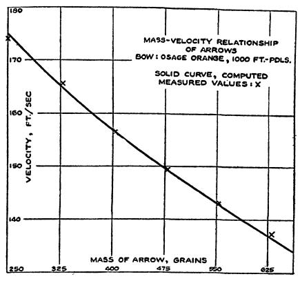
FIGURE 9.—Relation between mass of an arrow and its velocity when shot from a bow having 1,000 foot-poundals of available energy at full draw.
