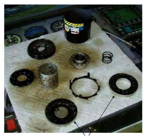
The folded paper filter element was between these two parts and was cut off with a carton cutter.
