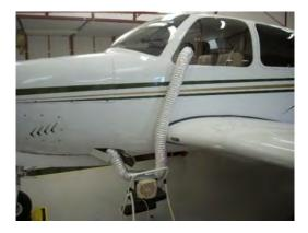
NOTE: I think if this were my design, I would just buy two of the heaters, one for inside the cabin and one with the duct work to heat the engine compartment. Then put the thing on a timer to automatically come on about an hour before you were going to be at the airport. Or as I mentioned above, use the light bulb under the engine and just leave it on all the time. And if your battery is not brand new, get a trickle charger and have it on in the winter time as well.
