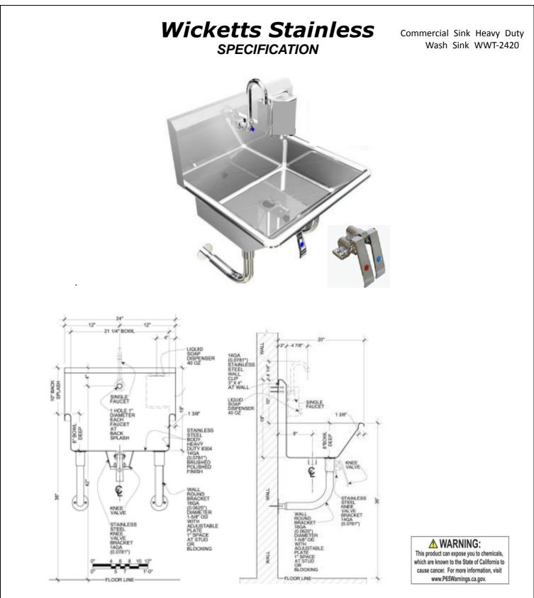
**Engineering Specification:** 14 gauge, type 304 stainless steel wash sink.1-3/8" rolled rim. 1-1/2" welded in drain. Exposed surfaces polished to a satin finish. Supported on (2) wall clips. Legs to wall.
