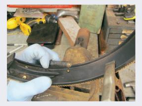
The brass partial hollow rivet head is now countersunk into the woven lining.
