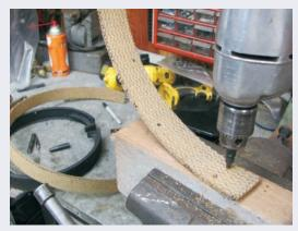
Now countersink each hole drilled on the outside face of the lining using the countersink portion of the bit. Only go half way deep, just enough to sink the rivet head into the lining and to have the solid barrel of the brass rivet just at the rim of the metal shoe band.
