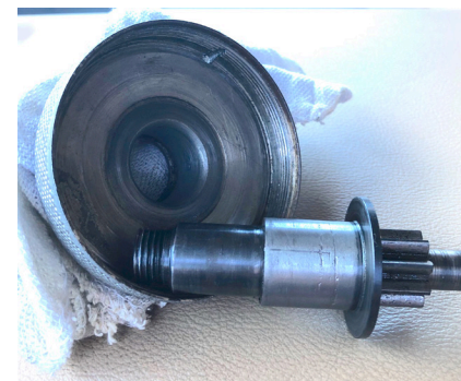
Re-worked steering case cover and steering pinion shaft
