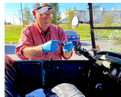
Installing pinion shaft into cluster, with lots of grease on shaft and cluster gears
