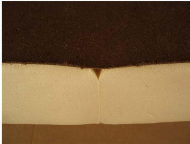
Knit line and V-groove close-up (after conditioning)
