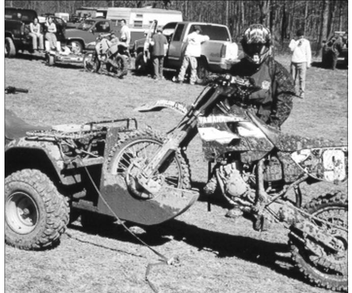
This is one of the neatest gadgets I've seen in a long time. One of the Razorback Rider club members made this tow system for hauling dead bikes out of the woods. He said that if a bike with a 19 inch front wheel needs to be pulled out, put a board in the bottom and another in the front and use the tie-downs, like any other bike. Since the bottom of it bolts to the trailer hitch and the top to the rack, the rear suspension of the ATV doesn't move. Every club needs one of these.
