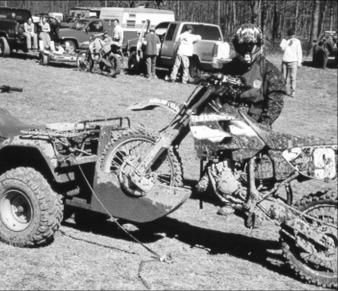
This is one of the neatest gadgets I've seen in a long time. One of the Razorback Rider club members made this tow system for hauling dead bikes out of the woods. He said that if a bike with a 19 inch front wheel needs to be pulled out, put a board in the bottom and another in the front and use the tiedowns, like any other bike. Since the bottom of it bolts to the trailer hitch and the top to the rack, the rear suspension of the ATV doesn't move. Every club needs one of these.
