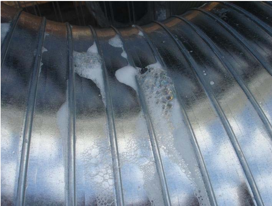
Figure 5 Picture of 19.3-inch (490 mm) Elbow during Soap Bubble Evaluation
