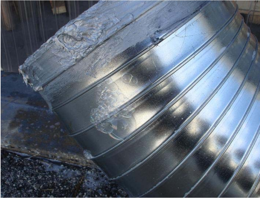
Figure 4 Picture of 15.6-inch (395 mm) Elbow during Soap Bubble Evaluation
