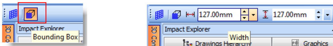
Fig 19 – 3D>New>Grid tool – with the 'Bounding Box' option enabled (left) and disabled (right)
