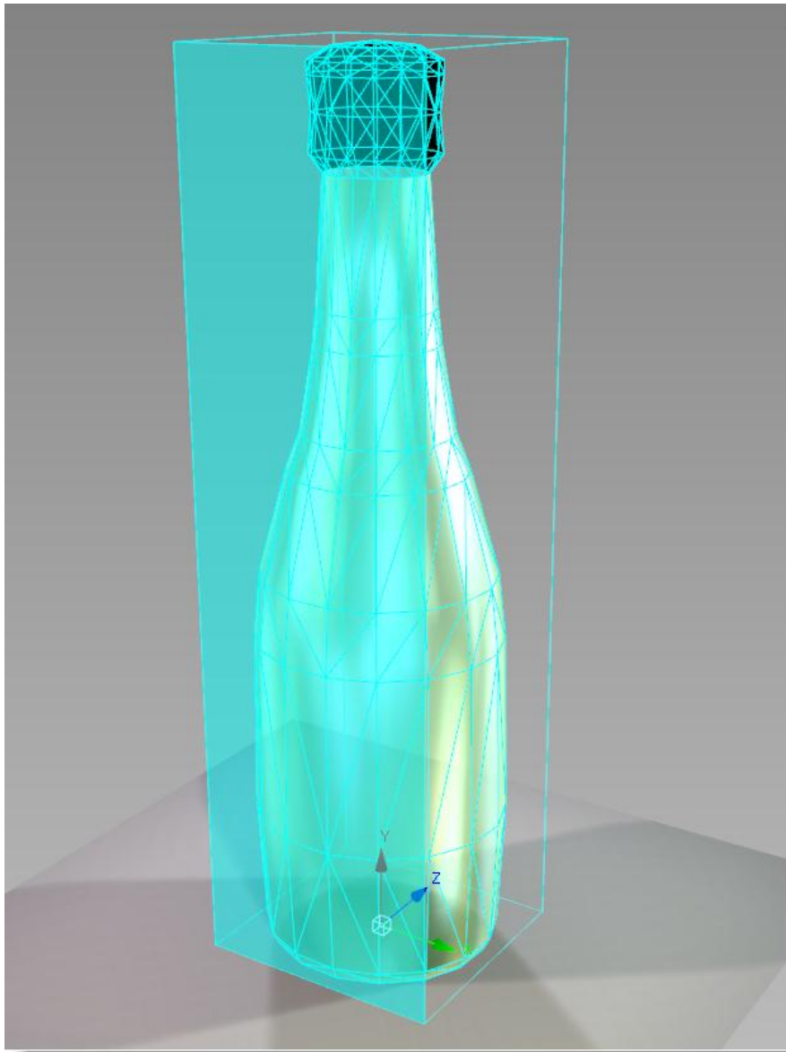
Fig 29 – Grid placement on realigned bounding box
