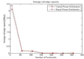
Figure 4.2 Average Cell Capacity of macrocell edge users.
