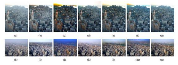
Fig. 10. Haze removal results by the algorithms in [7], [14], [27], [33], and [34] and the proposed algorithm. (a, h) input images; (b, i) de-hazed images by the algorithm in [34]; (c, j) de-hazed images by the algorithm in [27]; (d, k) de-hazed images by the algorithm in [33]; (e, l) de-hazed images by the algorithm in [7]; (f, m) de-hazed images by the algorithm in [14]; and (g, n) de-hazed images by the proposed algorithm.
