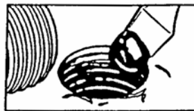
Step 5) Fill damage with FORM-A-THREAD™ compound.
