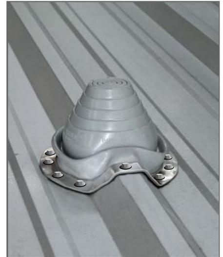
*Figure 9* Pipe Boots provide a water-tight seal around roof vents and come in a variety of sizes. They seal with caulk and conform to the shape of the panel ribs.
