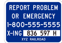
Emergency Notification Systems sign
