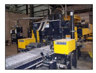
Cured block is processed through the block splitter. Block is inspected for specification conformity prior to being palletized and transferred the inventory storage area.
