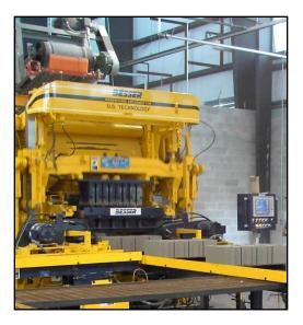
The mixture is fed into the block mold, vibrated to assure there are not any voids in the formed block and compacted to the final block shape.
