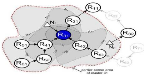
Fig.12 : The carrier-sense area and collision domain (bold routers) of cluster 31
