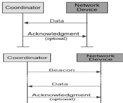
Fig.5: Acknowledgment Beacon network communication
