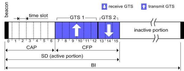
Fig.6: Super frame structure of IEEE 802.15.4.
