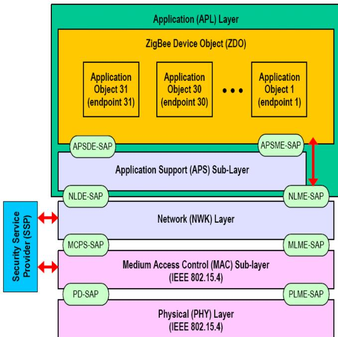
Fig.8: ZigBee Stack System Requirements
