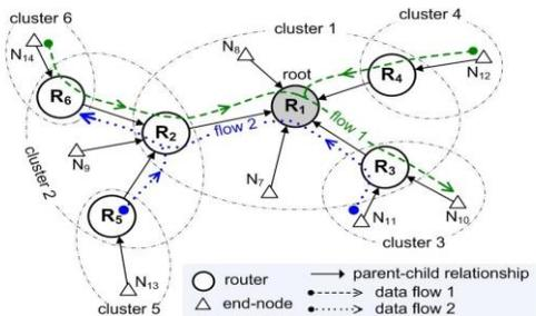
Fig.9: Cluster-tree topology with 2 time-bounded data flows.
