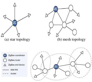
(c) cluster-tree topology Fig.7: IEEE 802.15.4/ZigBee network topologies
