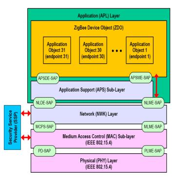
Fig.8: ZigBee Stack System Requirements
