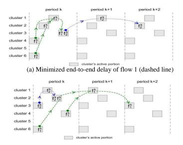
(b) Minimized end-to-end delay of flow 2 (dotted line) Figure 11: Schedules for data flows
