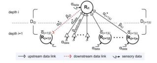
Fig.14: General data flow model with corresponding arrival and service curves.
