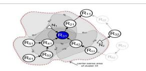
Fig.12 : The carrier-sense area and collision domain (bold routers) of cluster 31
