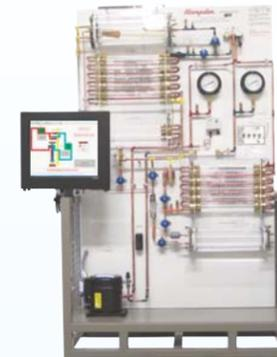
Hampden **H-RST-2-CDL-DEMO** Refrigeration System Trainer was designed to provide students with an actual working model of a refrigeration system, complete in every detail.
