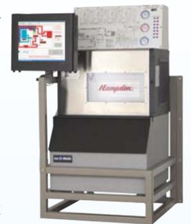
The unit consists of three sections: the ice cube machine, bin, and the control panel with six electrical and four mechanical programmable faults (optional). The ice cube machine has an efficient vertical plate design with positive release harvest assist. The foamed-in-place polyurethane insulated head and fan pressure control maintains proper gas temperature to maximize freezing and harvest cycles. The bin provides support and ice storage for the ice cube machine.
