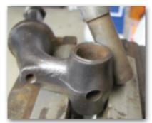
The fix is to replace the bushings. The chore is an easy home garage repair, as the only special tool that is nice to have is a bushing driver, sold by Model T vendors.
