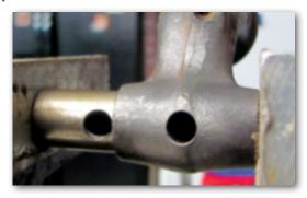
Therefore, after pressing in the new bushing, the hole must be reamed to allow the spring shackle to fit smoothly, but not tight. Use of a large twist drill (size 14.5 mm dia.) or similar reamer for the bushing allows for a nice fit.
