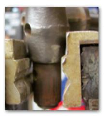
Fix the perch in a vise, or this can be done with the perch on the axle, too. Use a 5 lb. mallet and knock out the old bushing using the driver. Penetrating oil is helpful. (For a very stubborn bushing, a hack saw blade, in the bore to cut the bushing lengthwise, helps to ease removal.)
