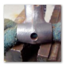
Once out, clean the bore of the perch and lightly oil to allow the new steel bushing to be driven in place with the tool, or use protected vise jaws to press the bushing in place.
