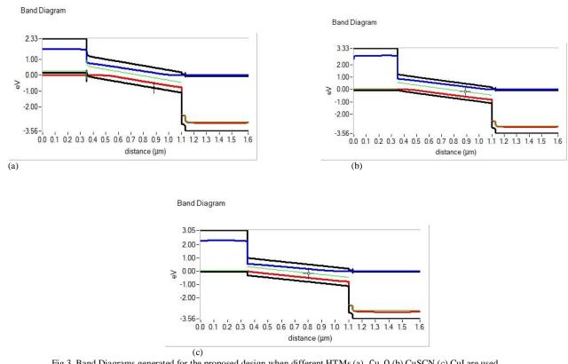
Fig 3. Band Diagrams generated for the proposed design when different HTMs (a) Cu<sub>2</sub>O (b) CuSCN (c) CuI are used
