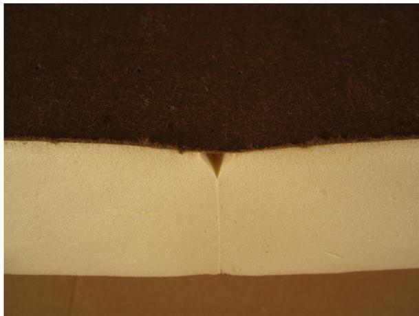
Knit line and V-groove close-up (after conditioning)
