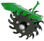
The CURVETINE CLOSING WHEEL “chips-in” the sidewall compaction often produced by the vee-opener blades. It crumbles the soil and promotes lateral root penetration. The pronounced curve allows the tine to ease out of the ground without ejecting material like a straight tooth closing wheel. The thumb-like tooth will firm and provide seed-to-soil contact. This makes moisture available and prevents the appearance of air pockets around the seed.
