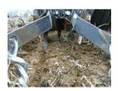
The Spading-Closing Wheel moves soil toward the seed at planting depth, while lifting and fracturing the surface layer to achieve compaction-free closing of the seed trench in wet, hard or sod conditions. With soil firmed around the seed from each side and the surface layer loosened, crops emerge sooner and planting can be done at the proper depth, even in wetter conditions, without fear of crushing the soil above the seed which would prevent emergence.
