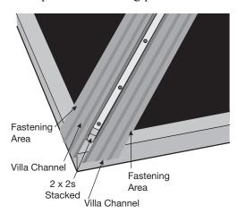
**Villa Valley:** Install Villa Valley or standard concrete valley metal (with same specifications as Villa Valley) along all valleys. All valley metal should be minimum 26 gauge pre-finished aluminum-zinc alloy coated steel. Valley metal should be a minimum 16" wide, with a minimum center upstand of 3-1/4". In new construction, the metal valley flashing must have one layer of Type 30 felt underlayment, 36" wide or ice & water shield underneath as required by local building code.
