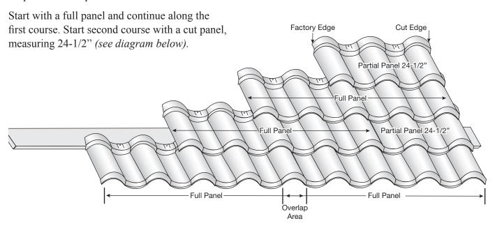
Measure panels and make cuts accordingly so the cut edge starts (or terminates) in the Villa Channel or Villa Valley (see diagram below). Panels can be cut from either side (see diagram right). Save cut-off pieces for use on opposite side terminating into Villa Valley or Villa Channel.
