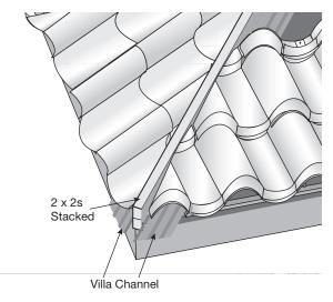
Panel Installation - Valley: When installing Villa Panels along the valleys, the panels will terminate into the Villa Valley. See Villa Valley Section (page 6) for installation of Villa Valley and preparation prior to installing panels. Measurements for valley cuts are made much like the hip cuts. Measure and cut the panels carefully so they fit tight against the Villa Valley. If a cut-out panel at the valley is too small, lap over two pans to allow proper fastening.
