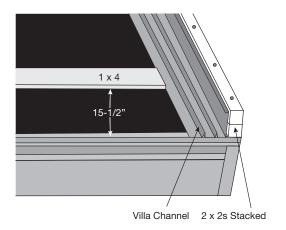
**Panels - First Course:** Fasten the first course of panels through the pre-punched fastening tabs to the 1 x 4s using minimum #9 Hex (1/4" diameter) x 1-1/2" long screws that will fit flush to panel and are long enough to penetrate the deck securely.
