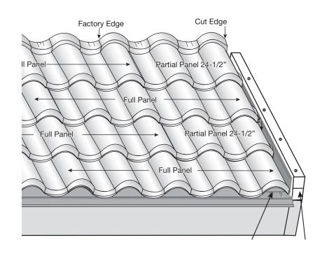
Pre-paint vertical/exposed portion of Villa Channel & Valley prior to installing panels.
