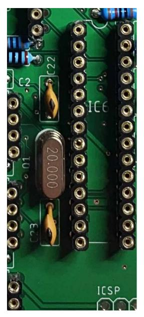
Install and solder the thirteen 100nf capacitors C1, C2, C3, C4, C5, C6, C7, C14, C15, C16, C17, C18, C24.
