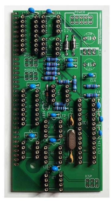
Cut three pieces of 2x3 male pin headers and install and solder into ICSP, MIDIIN and MIDIOUT.
