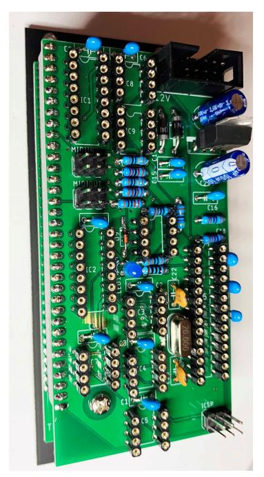
Install the 6N138 opto coupler into OK1.
