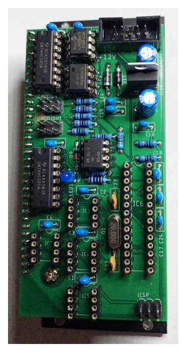
Install the four MCP602 ICs into IC3, IC4, IC5 and IC7.
