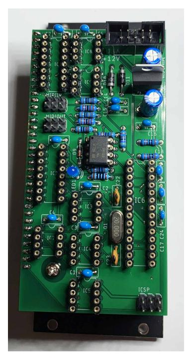
Install the MCP4822 DAC into IC8.
