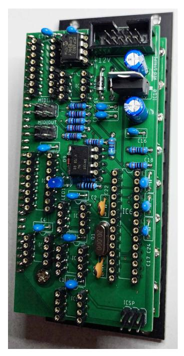
Install the TL072 IC into IC9 and the two 74HC595 ICs into IC1 and IC2.
