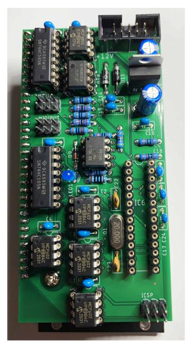
Lastly install the ATMega328 IC into IC6.
