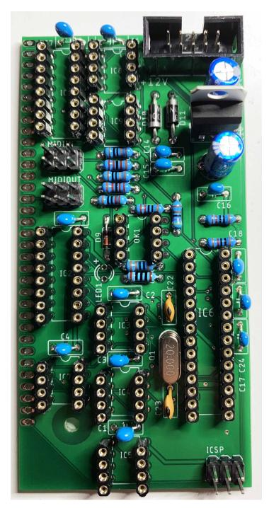
Install and solder LED1 paying attention to the + symbol on the PCB which is the long pin of the led.
