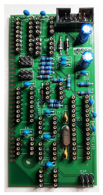
Install and solder the one 7805 voltage regulator into IC10.
