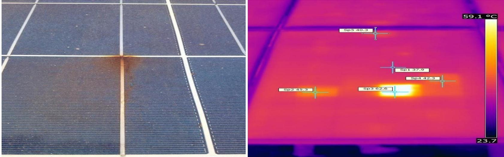
**Module O/P with Cell burnt module**
