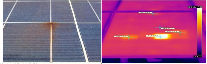
Module O/P with Cell burnt module
