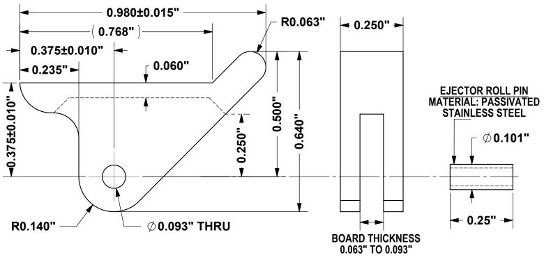
Once the ejector is installed, proper adjustment of the board in relation to the card guides will influence the effectiveness of the ejector. The ejector must have a surface to bear against within 0.150" of the edge of the board. The ejector lever arm must rest on this surface. If the card is pushed deeper into its card guides the ejector will lose its mechanical advantage.
