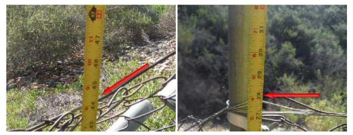
\* The minimum California safety building code requires safety barrier fencing for pools with spas to be a minimum of 60-inch high from grade level (on both sides of the fencing) and completely around the yard with the pool with spa in order to control unsupervised access to the pool or spa waters, which, historically have had horrific consequences. The less than minimum 60-inch high safety barrier fencing is a **SAFETY HAZARD CONDITION**.
