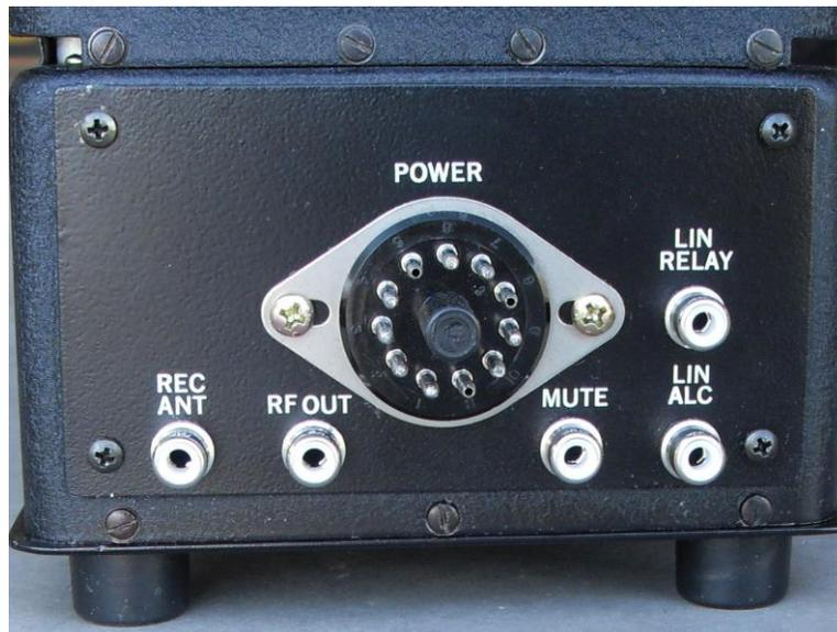
**Figure 2 – Rear Panel Connections**
