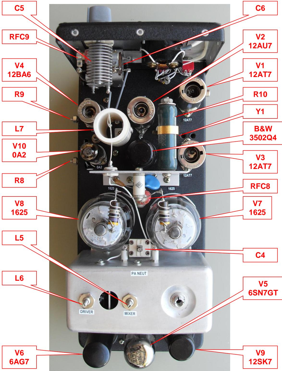
Figure 5 – Chassis Top View
